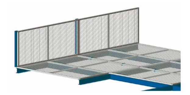
A distinction is made with respect to the fall protection panels between floor elements & side protection.
